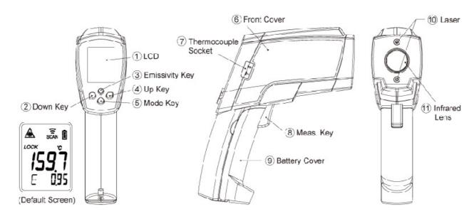
Simply aim the thermometer at the measure target with Lens (11) and press Meas. key (8) to display the surface temperature. The Distance:Spot is 75:1. The two laser points are the reference for the target spot size. Please make sure the target area is within the field of view.
